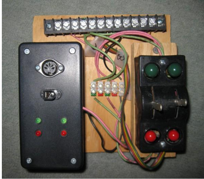
Figure 33: Example of opto-isolators used for Switch Direction Sensing
