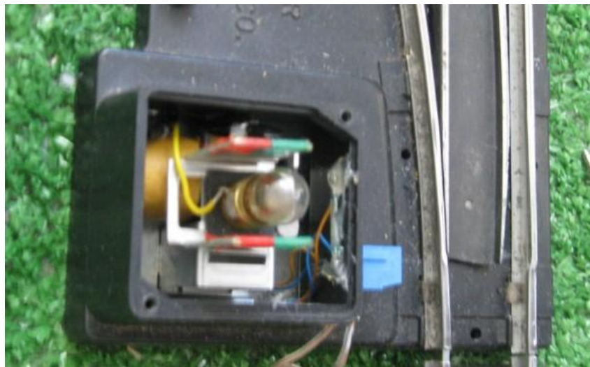
Figure 36: Example of magnetic reed switch used for Switch Direction Sensing
