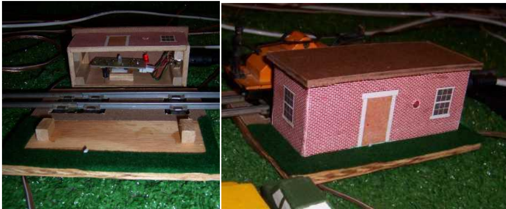
Figure 29: Reflective IR trip installed in track-side building
