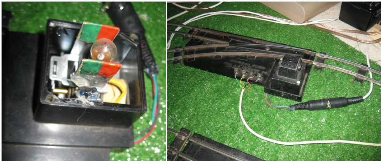
Figure 38: Example of hall effect sensor used for Switch Direction Sensing
