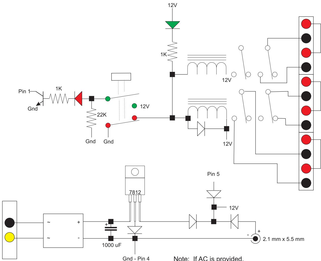
Note: If AC is provided, then it will take priority over the other two inputs, assuming the DC in will be less than 12.6 volts.
