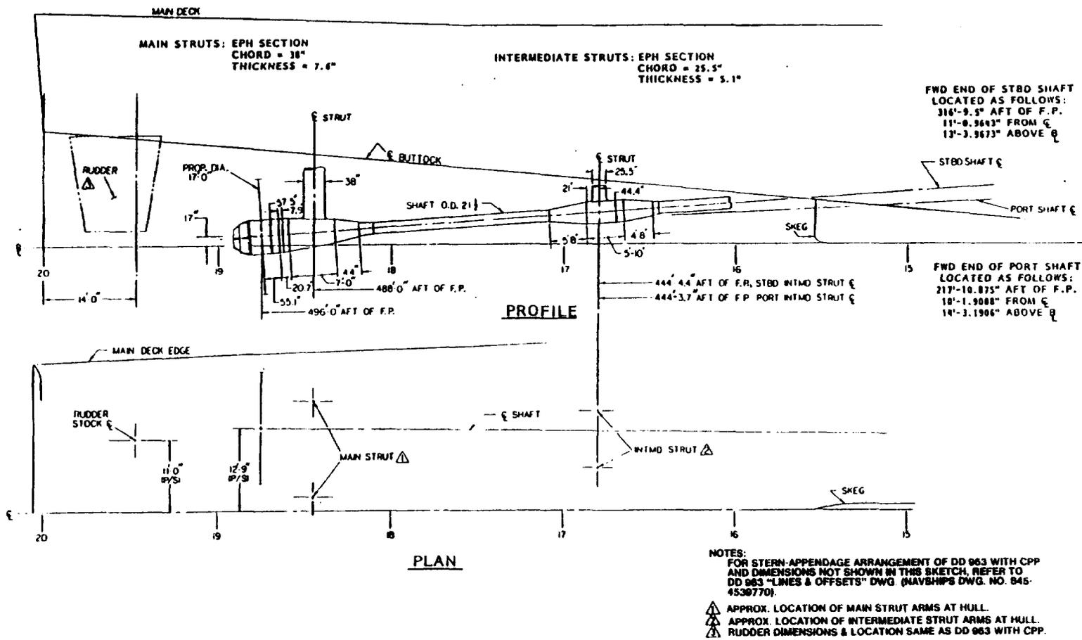
Figure A-1.6 - Stern Appendages of Parent Configuration, Twin Shafts and Struts with Controllable-Pitch Propellers - Profile and Plan Views, from Tomassoni and Slager (1980)
