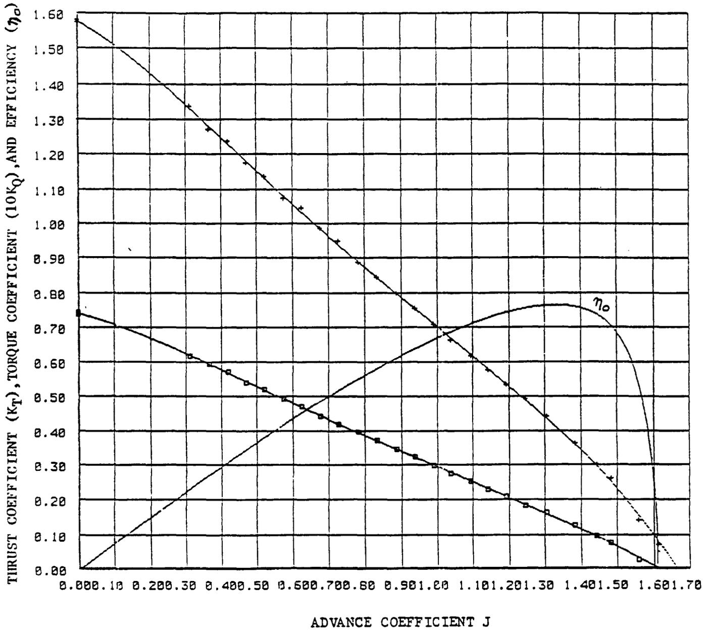
Figure A-5.3 - Open Water Curves for Propeller 4864
