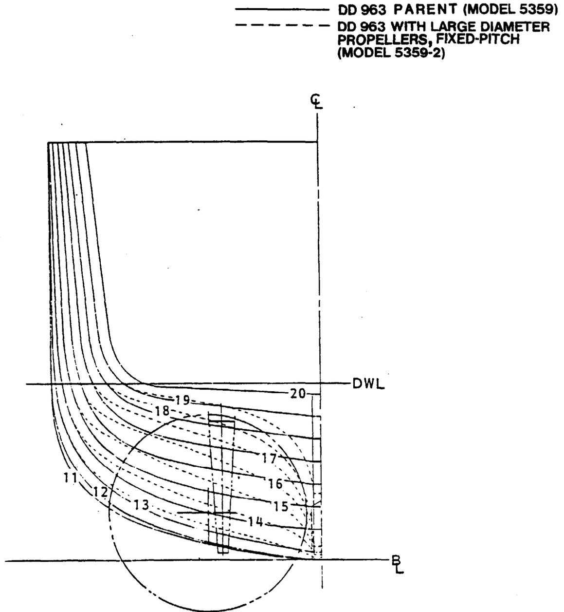
Figure A-7.4 - Comparison of Afterbody Sections of the Large Diameter Low Tip Clearance Propeller Configuration with Those of the Parent DD-963 Configuration, from Tomassoni and Slager (1980)
