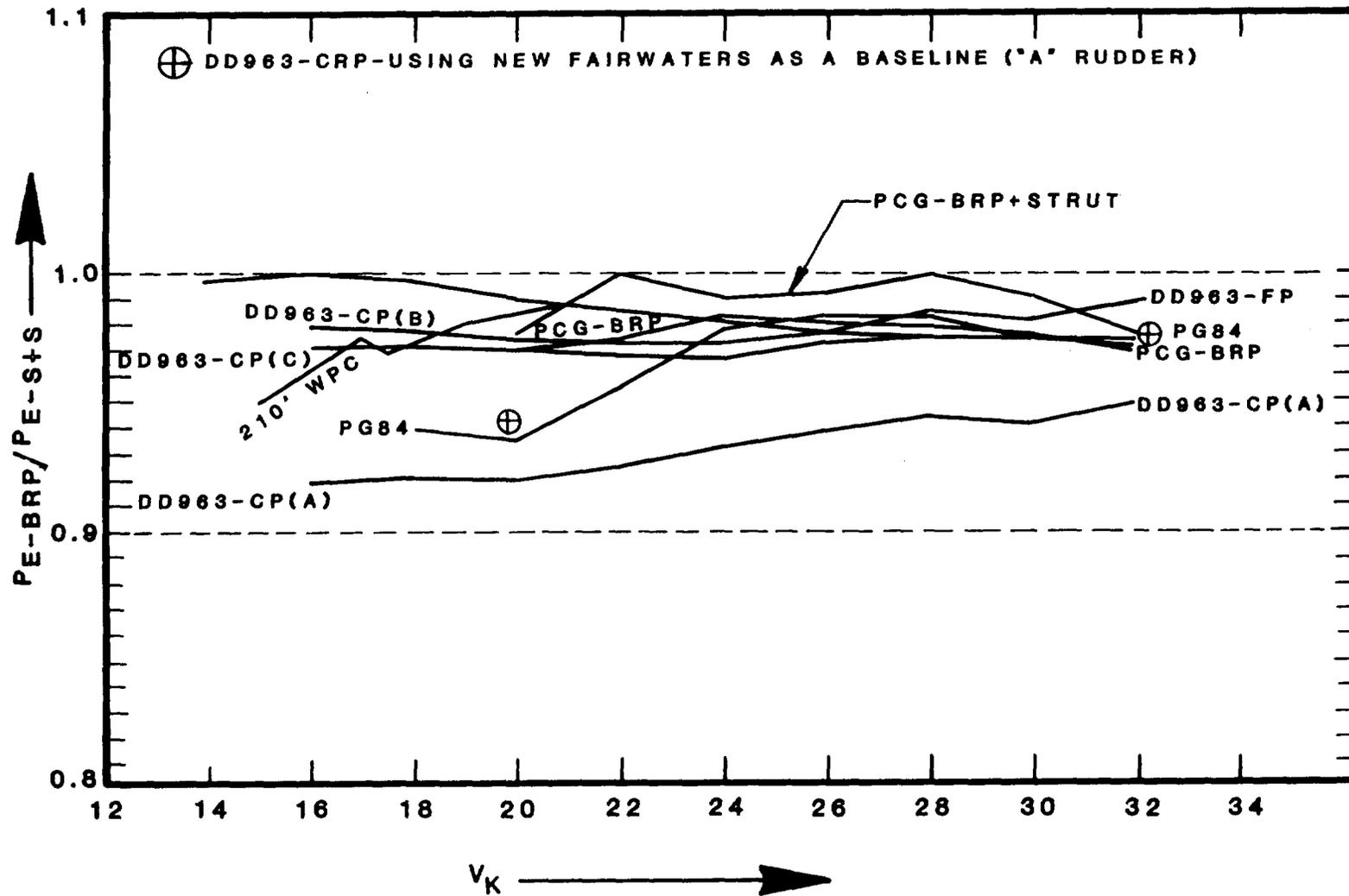
Figure E-2 - Comparison of Effective Power with Bearing-in-Rudder Post to that with Shafts and Struts for Seven Models, as a Function of Speed
