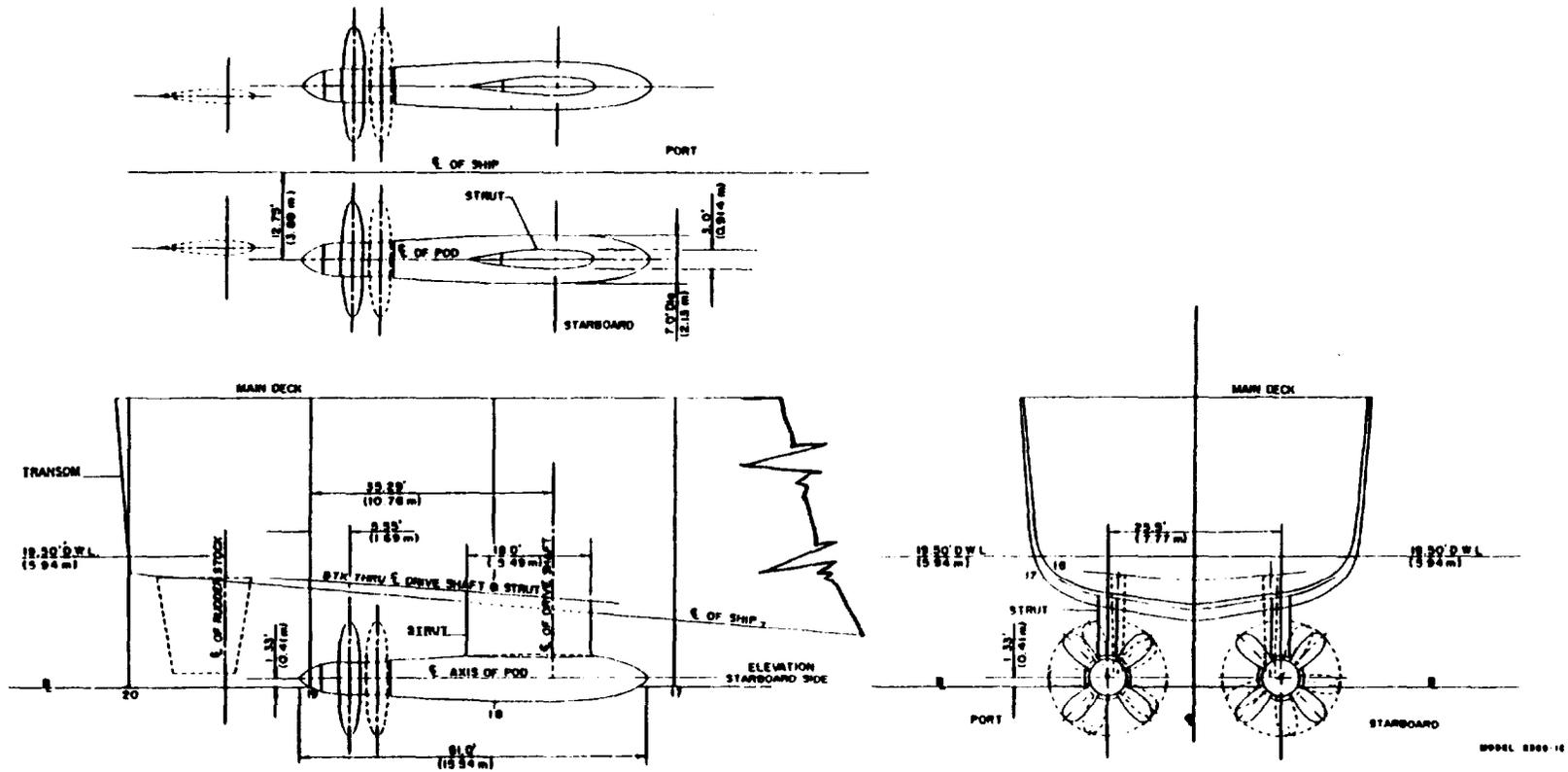
Figure A-2.4 - Form and Dimensions of Twin Pods with Contrarotating Propellers Fitted on DD-963 Hull Form, Represented by Model 5359-1C
