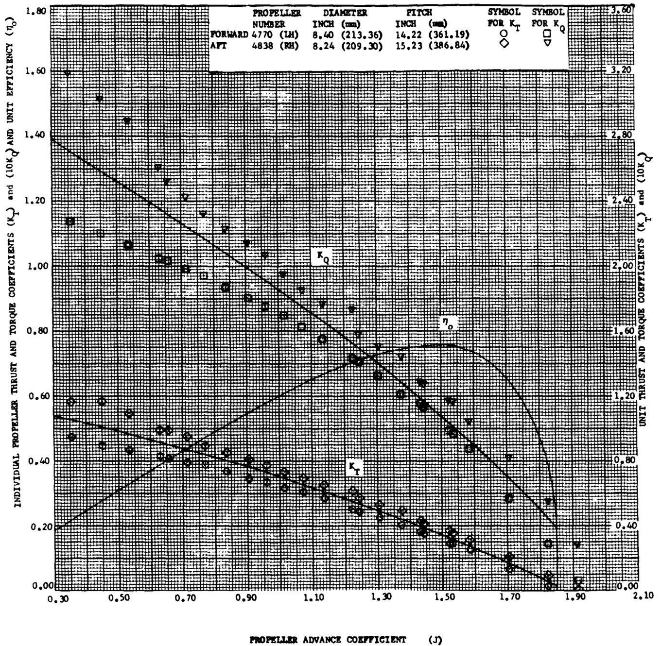
Figure A-2.3 - Open Water Curves for Contrarotating Propellers 4770 and 4838
