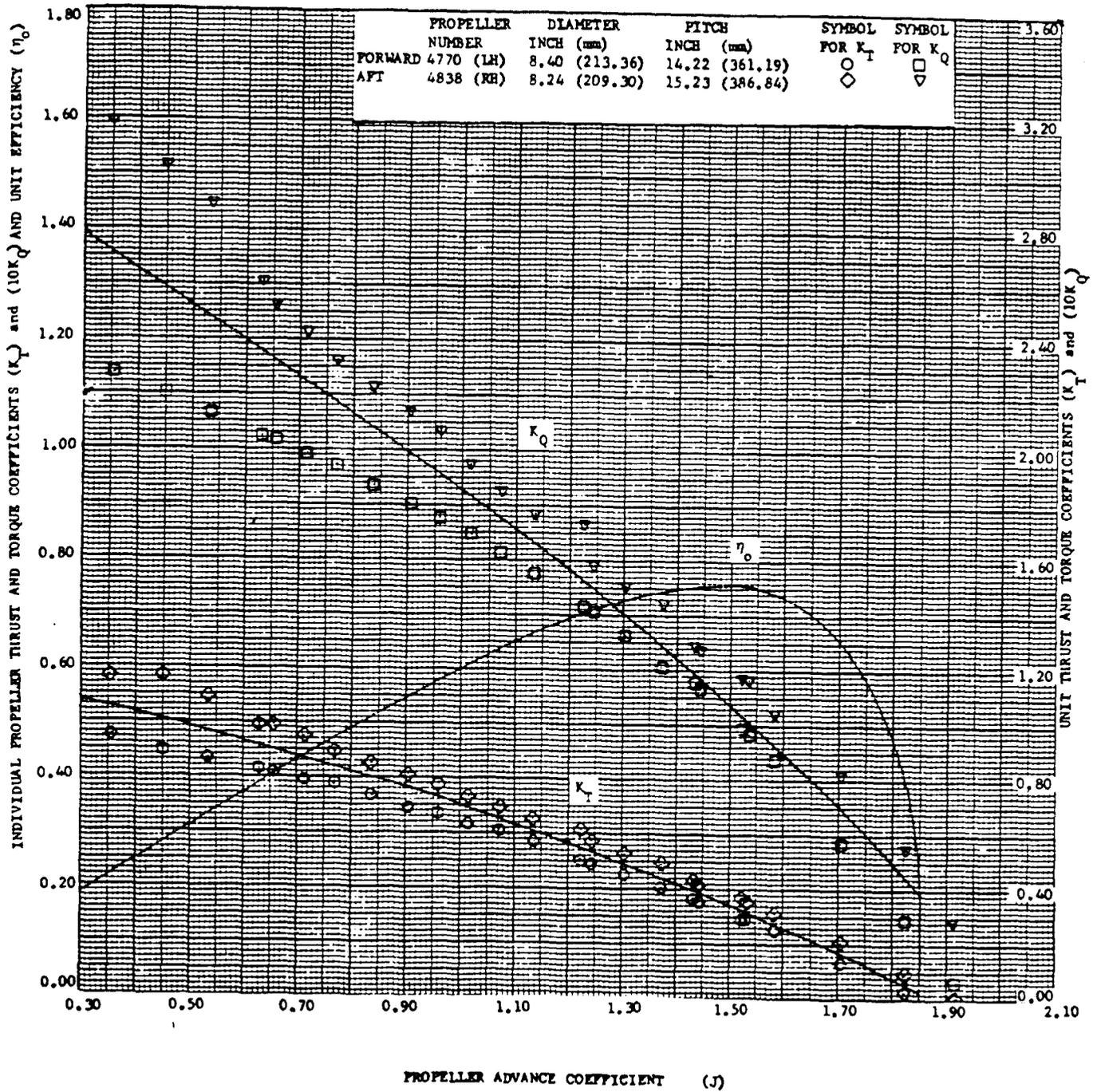
Figure A-4.2 - Open Water Curves for Contrarotating Propellers 4770 and 4838
