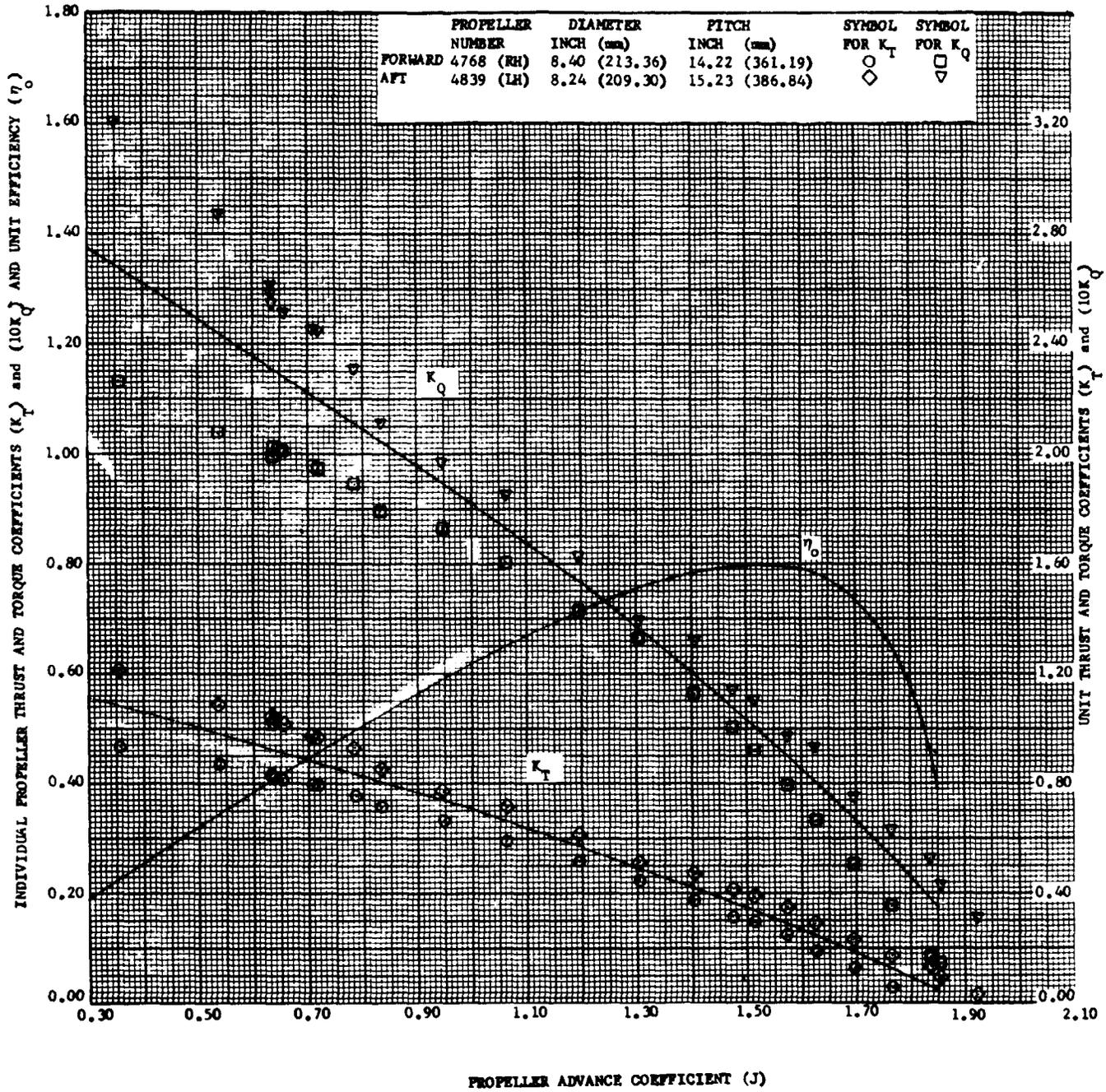
Figure A-2.2 - Open Water Curves for Contrarotating Propellers 4768 and 4839
