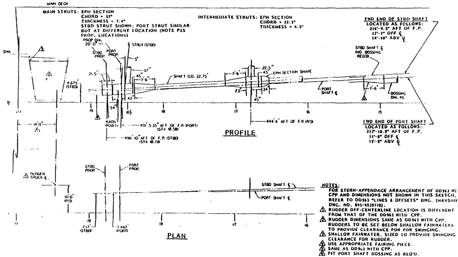
Figure A-10.5 - Stern Appendages of Large Diameter Overlapping Propeller Configuration - Profile and Plan Views, from Tomassoni and Slager (1980)
