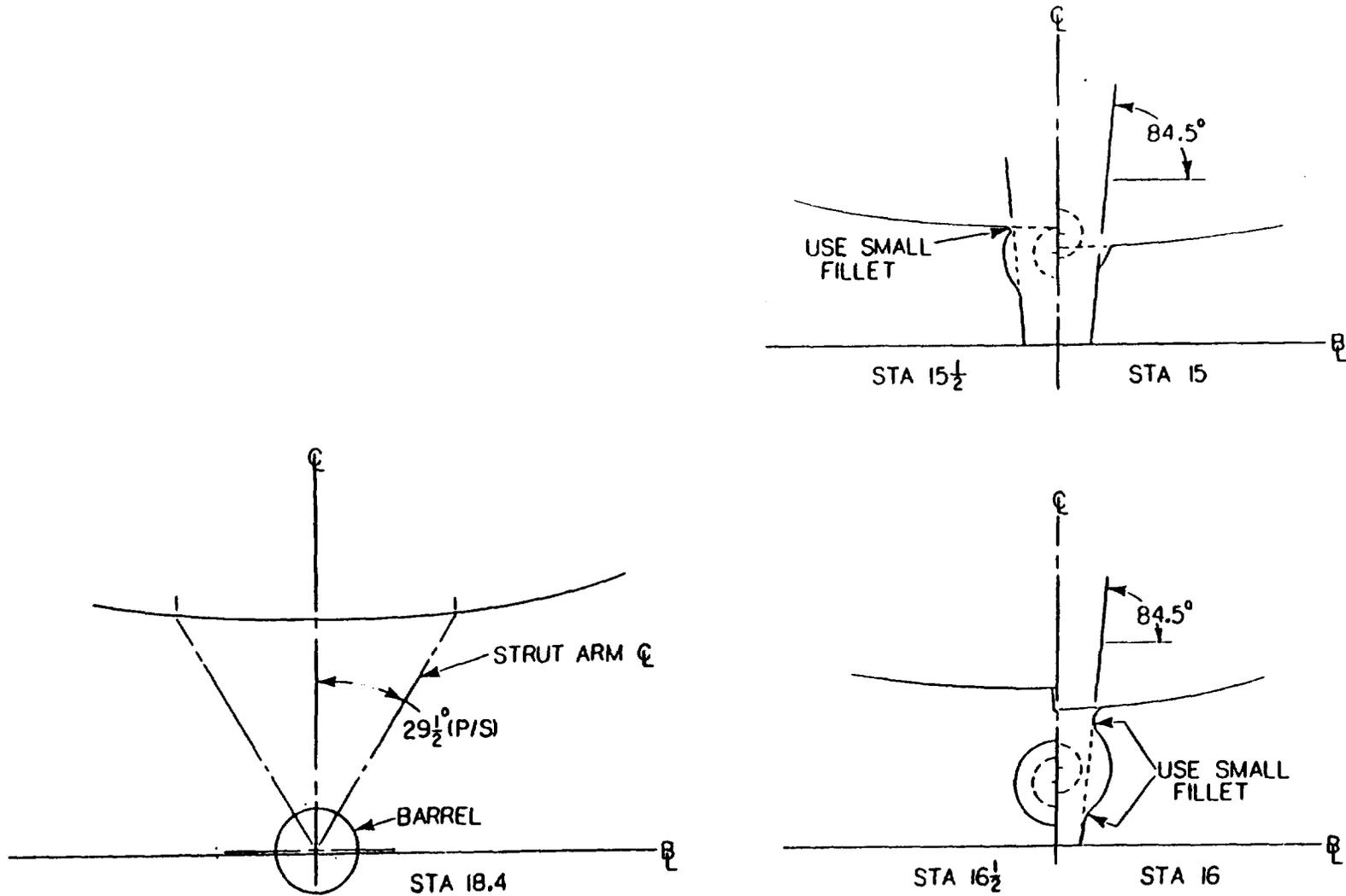
Figure A-13.4 - Stern Appendages of Single Shaftline Tandem Propeller Configuration - Sectional Views, from Tomassoni and Slager (1980)
