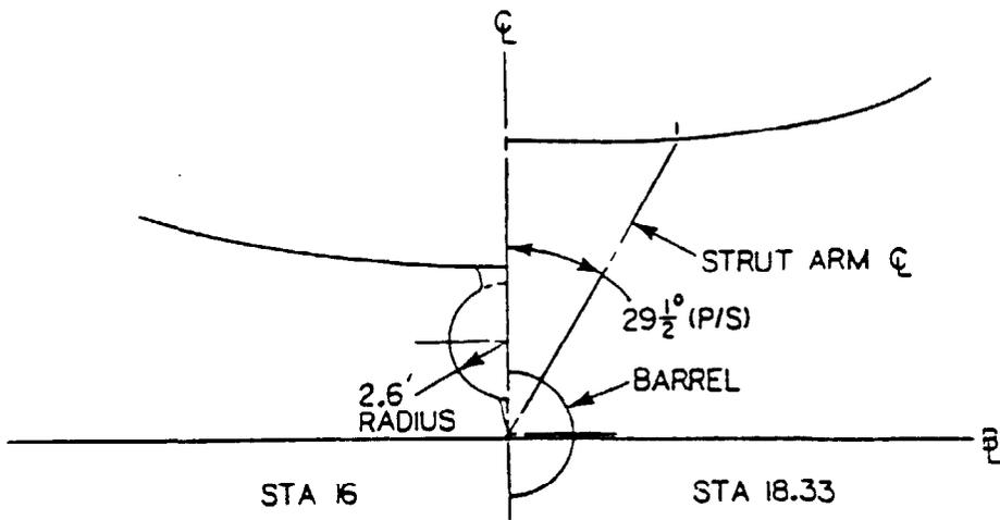
Figure A-12.6 - Stern Appendages of Single Shaftline Contrarotating Propeller Configuration - Section Views, from Tomassoni and Slager (1980)
