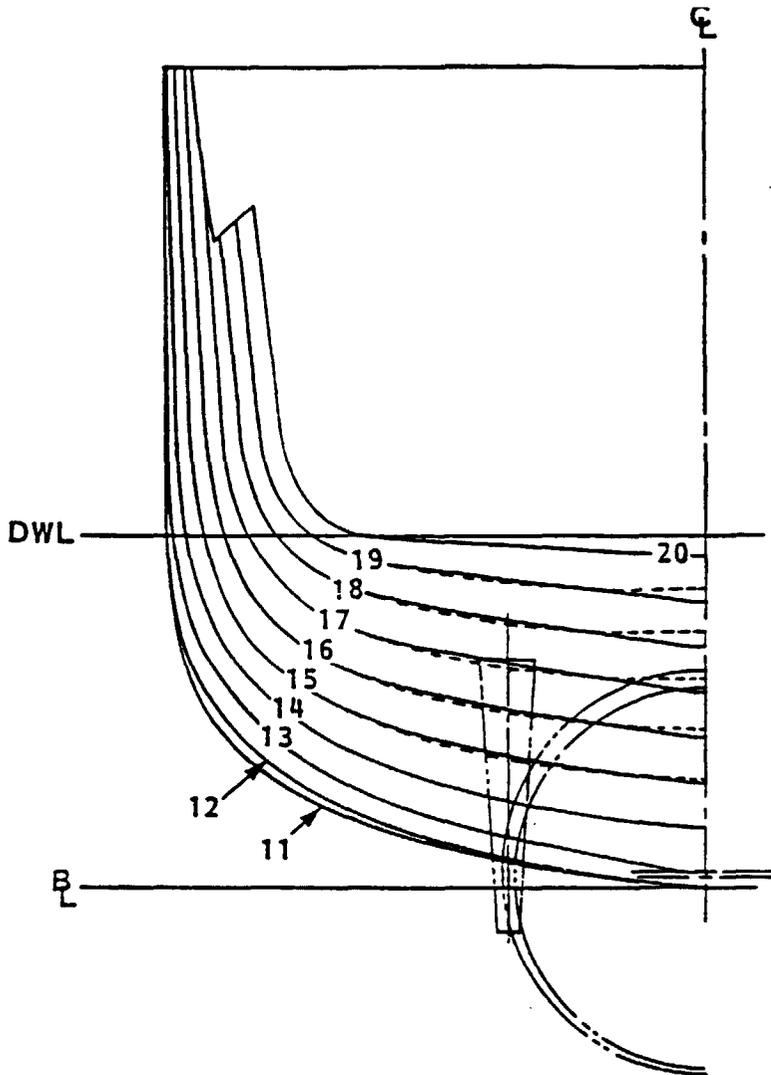
Figure A-12.4 - Comparison of Afterbody Sections of the Single Shaftline Contrarotating Propeller Configuration with Those of the Parent DD-963 Configuration, from Tomassoni and Slager (1980)
