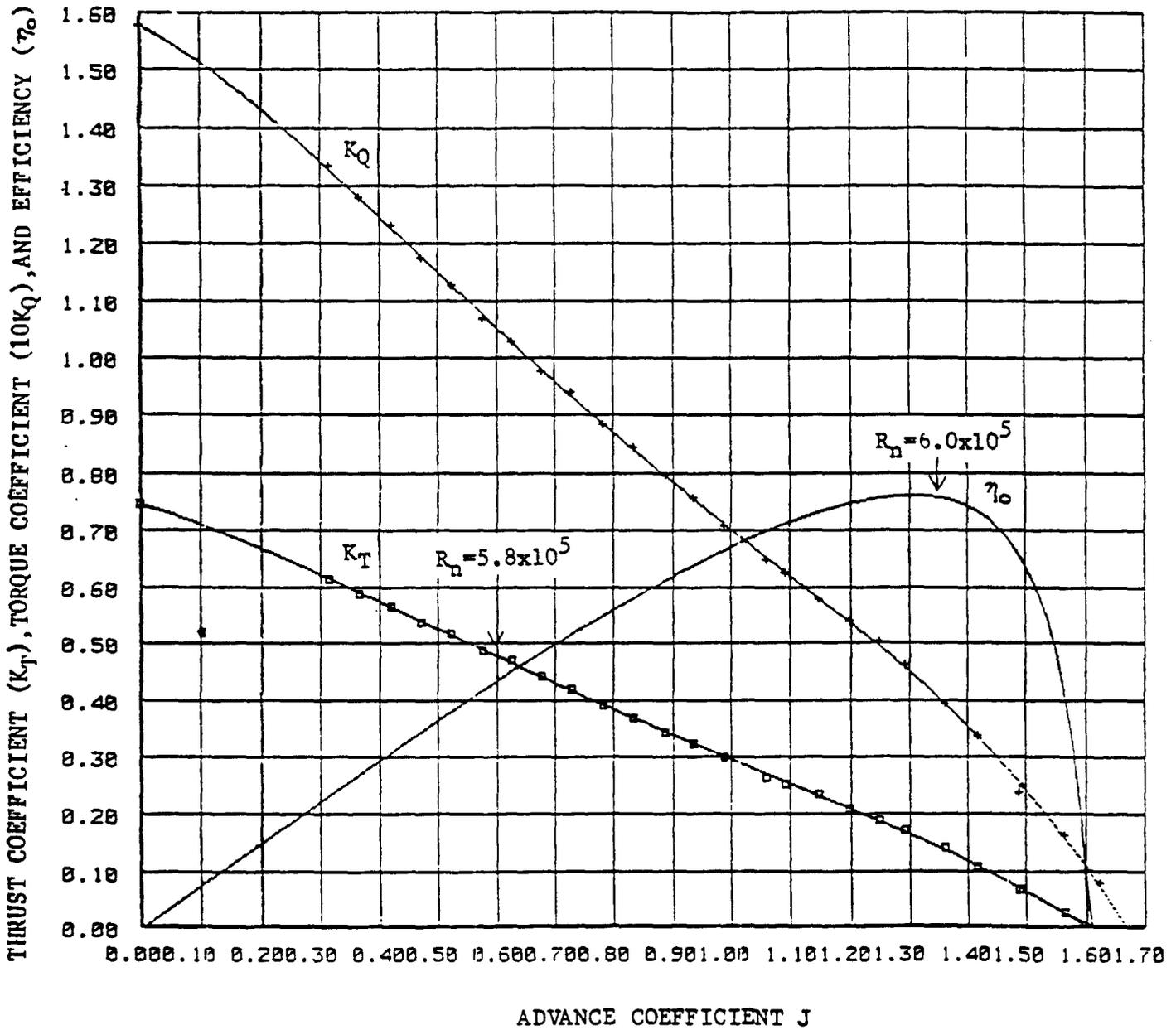
Figure A-5.2 - Open Water Curves for Propeller 4865
