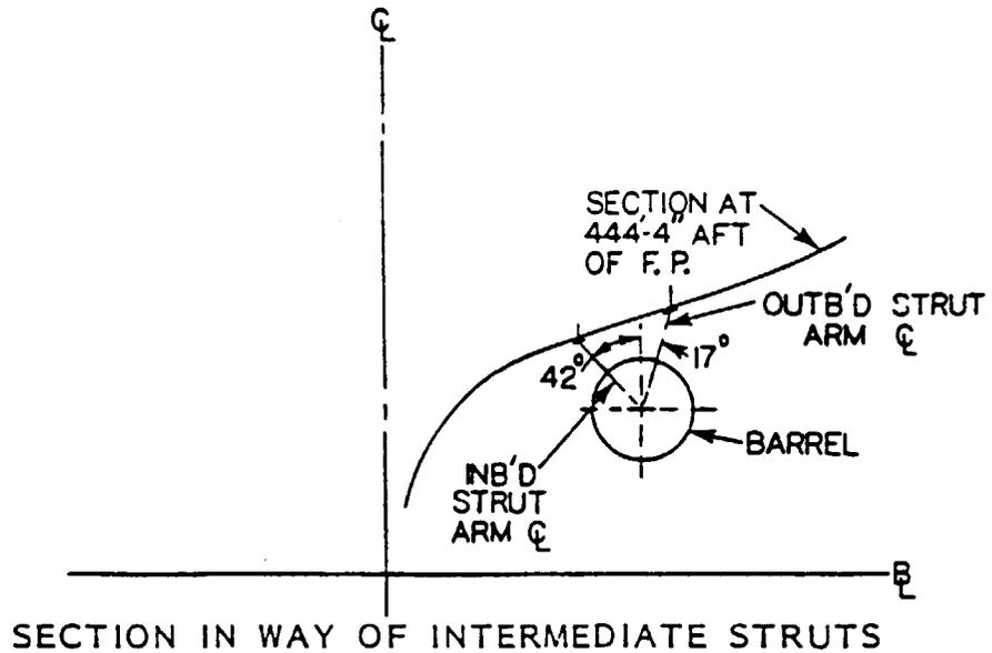
SECTION IN WAY OF INTERMEDIATE STRUTS
