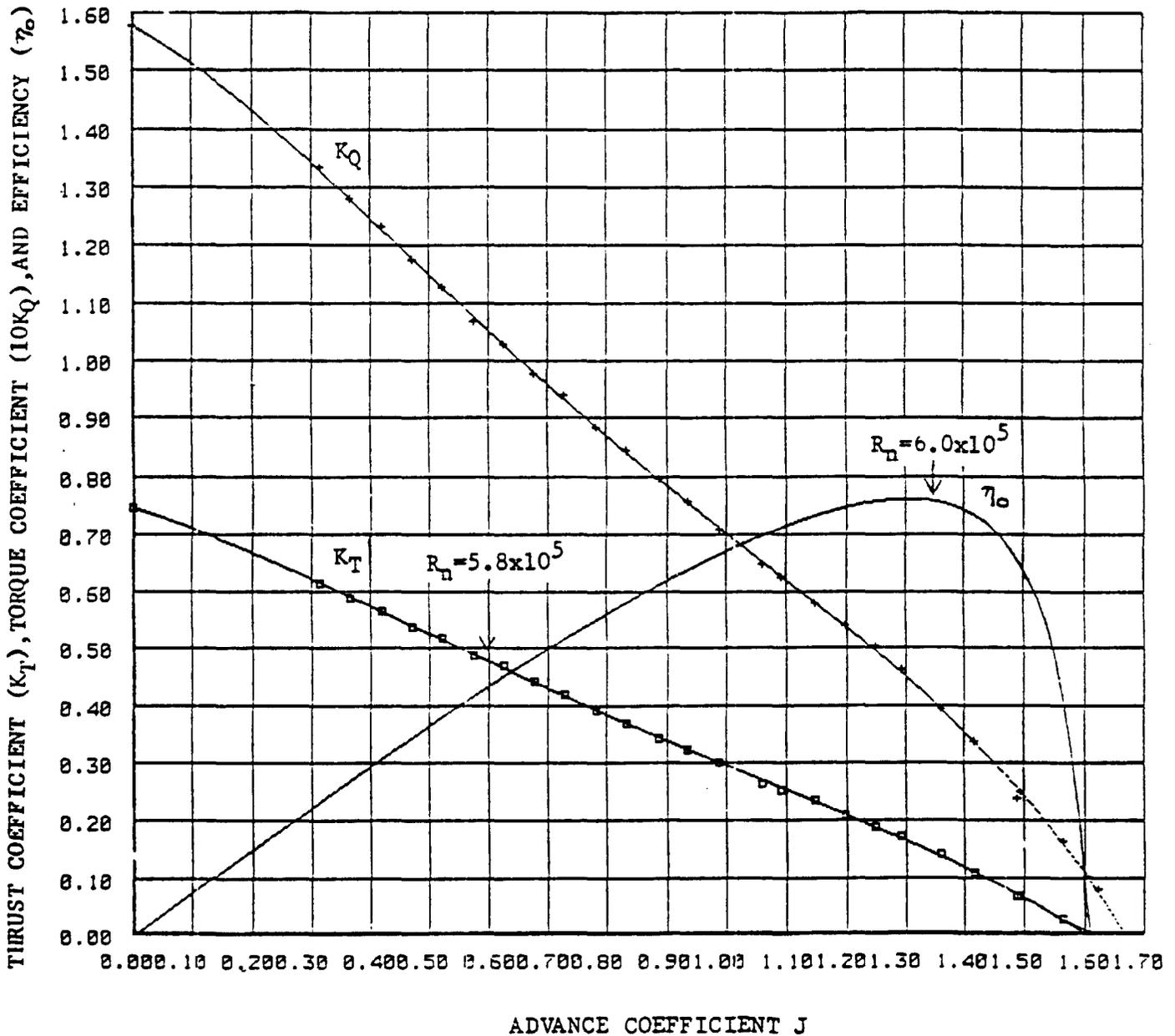
Figure A-3.3 - Open Water Curves for Propeller 4865
