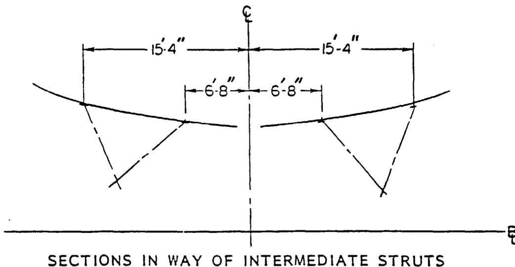
Figure A-8.4 - Stern Appendages of Twin Shafts and Struts Configuration with Tandem Propellers - Sectional Views, from Tomassoni and Slager (1980)
