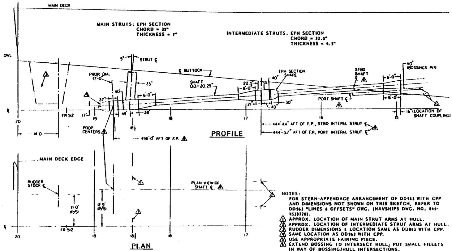
Figure A-5.4 - Stern Appendages of Twin Shafts and Struts Configuration with Fixed-Pitch Propellers - Profile and Plan Views, from Tomassoni and Slager (1980)
