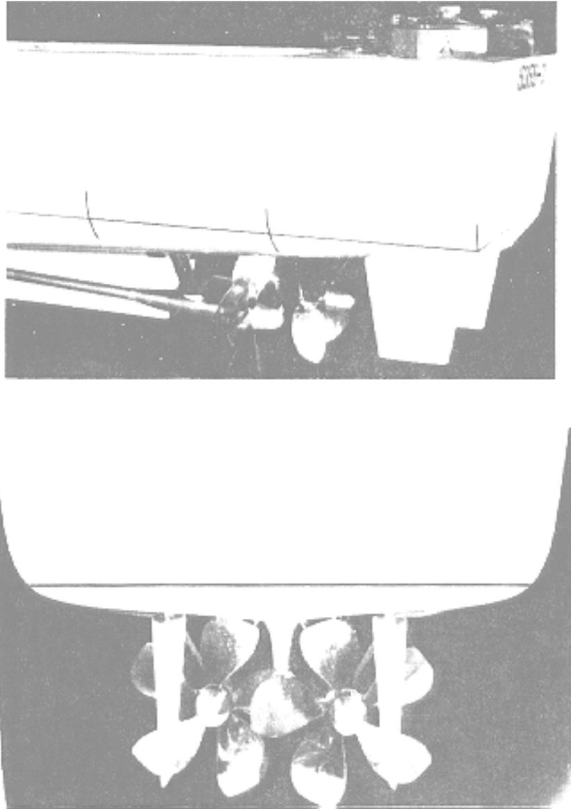
Figure A-10.7 - Photographs of Large Diameter Overlapping Propeller Configuration (Model 5359-3) - Stern Quarter and Stern View
