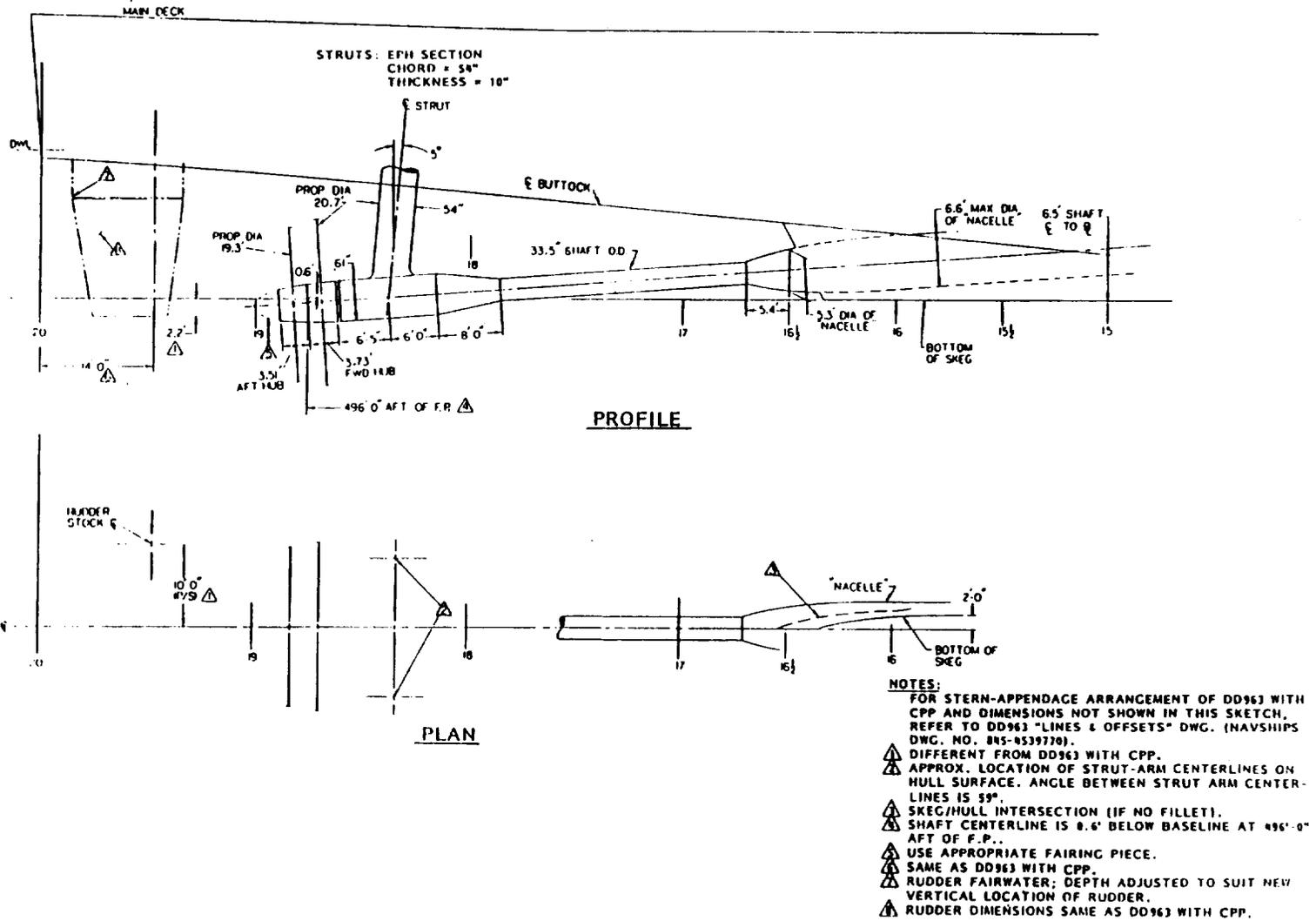
Figure A-13.3 - Stern Appendages of Single Shaftline Tandem Propeller Configuration - Profile and Plan Views, from Tomassoni and Slager (1980)
