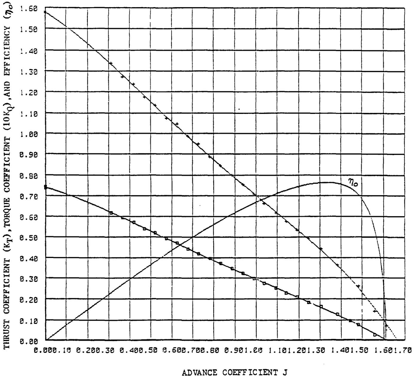
Figure A-3.2 - Open Water Curves for Propeller 4864
