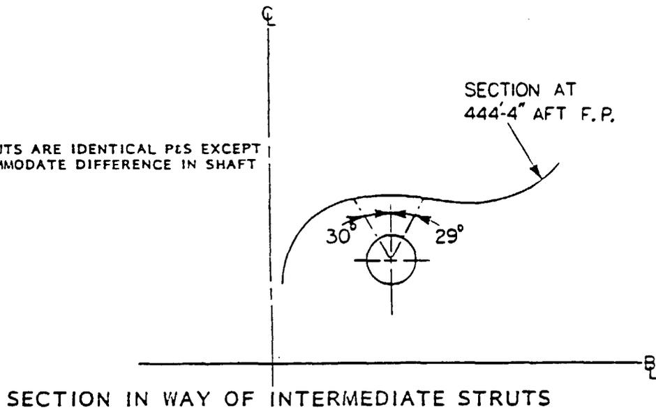
Figure A-10.6 - Stern Appendages of Large Diameter Overlapping Propeller Configuration - Sectional Views, from Tomassoni and Slager (1980)
