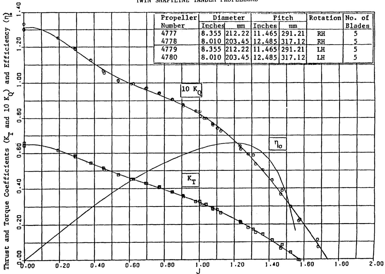
Figure A-8.2 - Open Water Curves for Tandem Propellers 4777 & 4778 and 4779 & 4780
