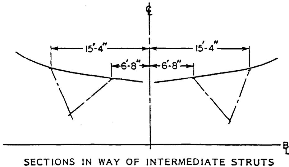
Figure A-1.7 - Stern Appendages of Parent Configuration, Twin Shafts and Struts with Controllable-Pitch Propellers - Sectional Views - Model 5359, from Tomassoni and Slager (1980)
