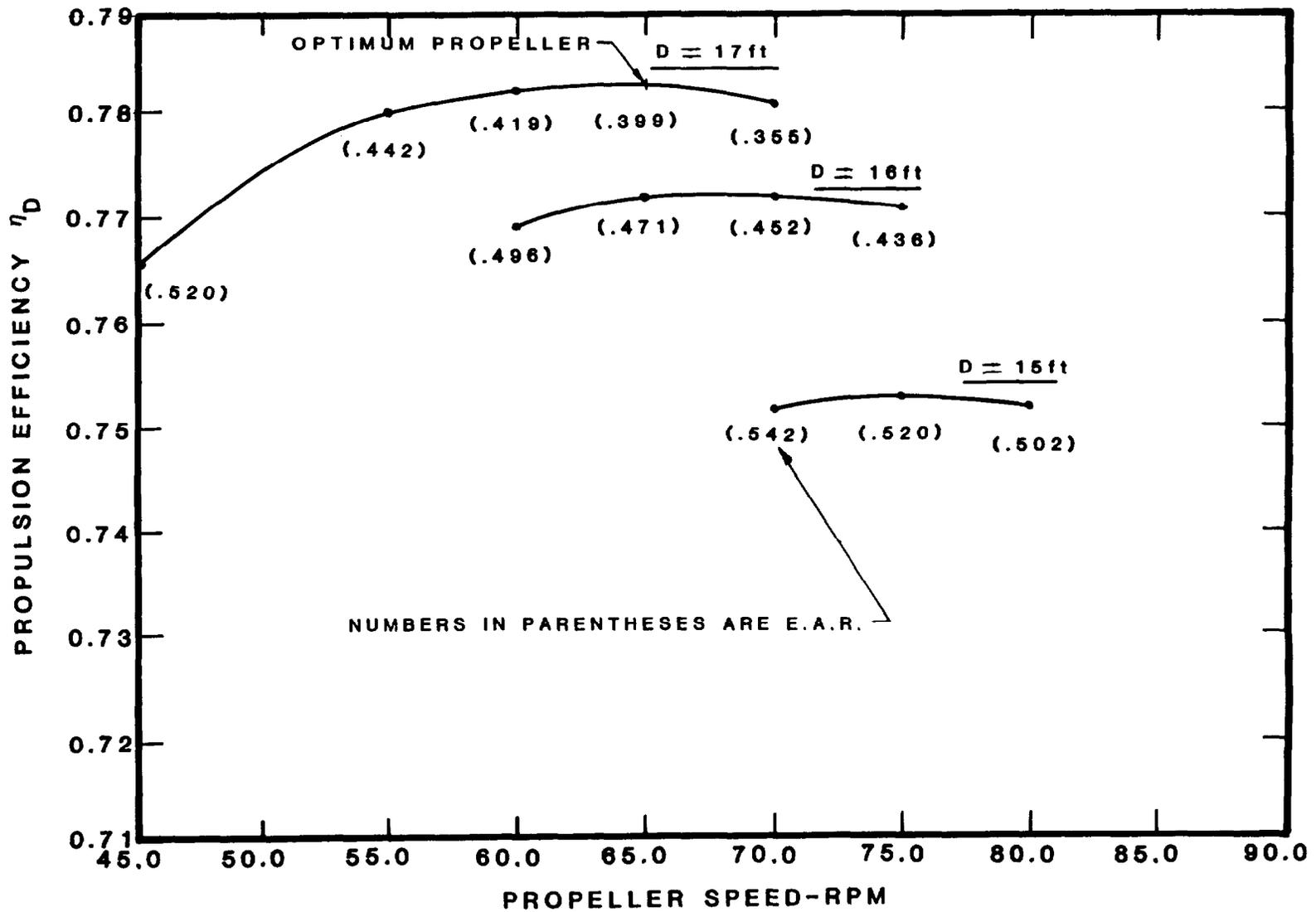
Figure C-1 - Propulsion Efficiency for Contrarotating Propellers on Twin Pods: Results of a Parametric Study
