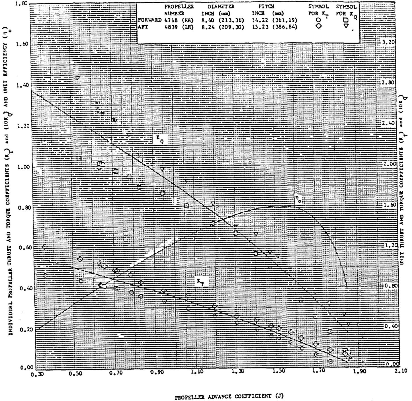
Figure A-4.3 - Open Water Curves for Contrarotating Propellers 4768 and 4839
