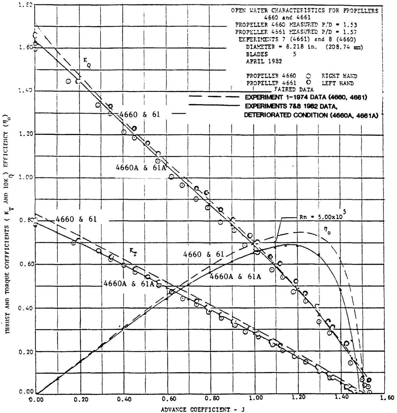
Figure A-6.2 - Open Water Curves for Propellers 4660A and 4661A in a Deteriorated Condition
