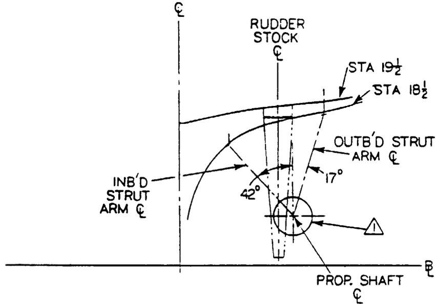
SECTION IN WAY OF MAIN STRUTS & RUDDERS
