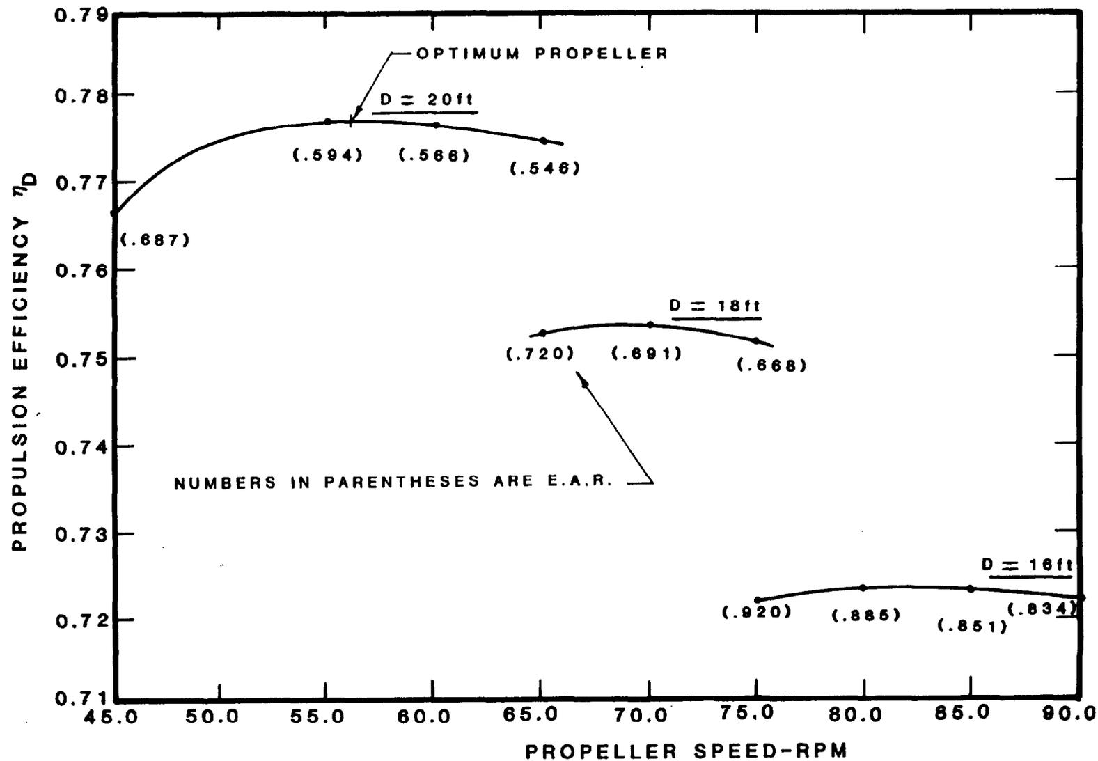
Figure C-3 - Propulsion Efficiency of Single Shaftline Contrarotating Propellers: Results of a Parametric Study
