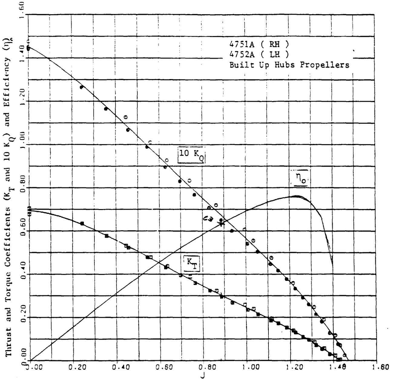
Figure A-11.2 - Open Water Curves for Propellers 4751A and 4752A
