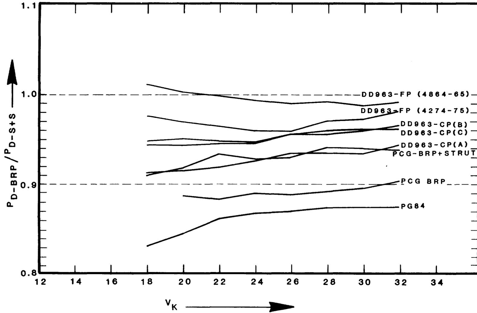
Figure E-3 - Comparison of Delivered Power with Bearing-in-Rudder Post to that with Shafts and Struts for Eight Models, as a Function of Speed
