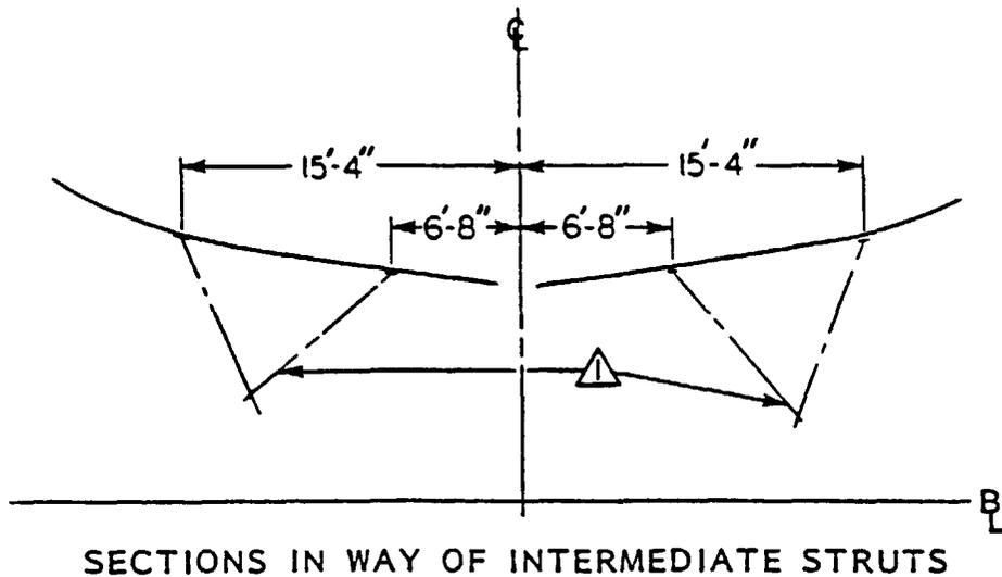
Figure A-5.5 - Stern Appendages for the Twin Shafts and Struts Configuration with Fixed-Pitch Propellers - Sectional Views, from Tomassoni and Slager (1980)
