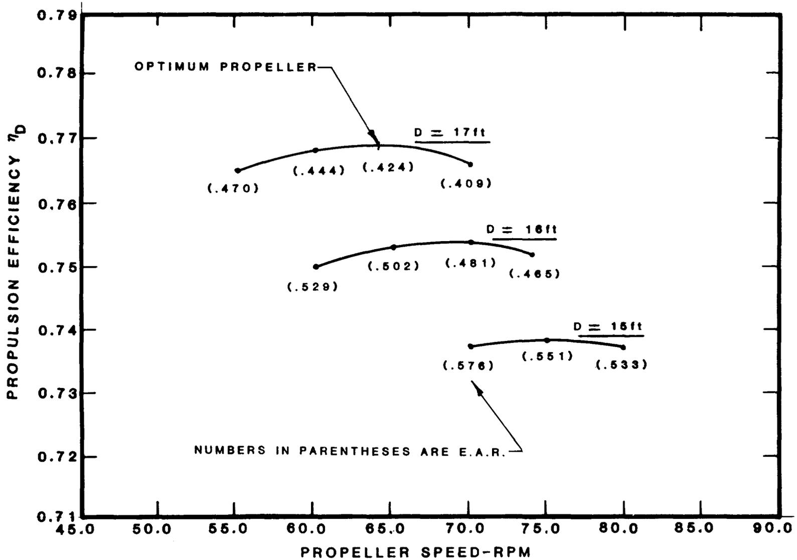
Figure C-2 - Propulsion Efficiency of Twin Shaftline Contrarotating Propellers: Results of a Parametric Study
