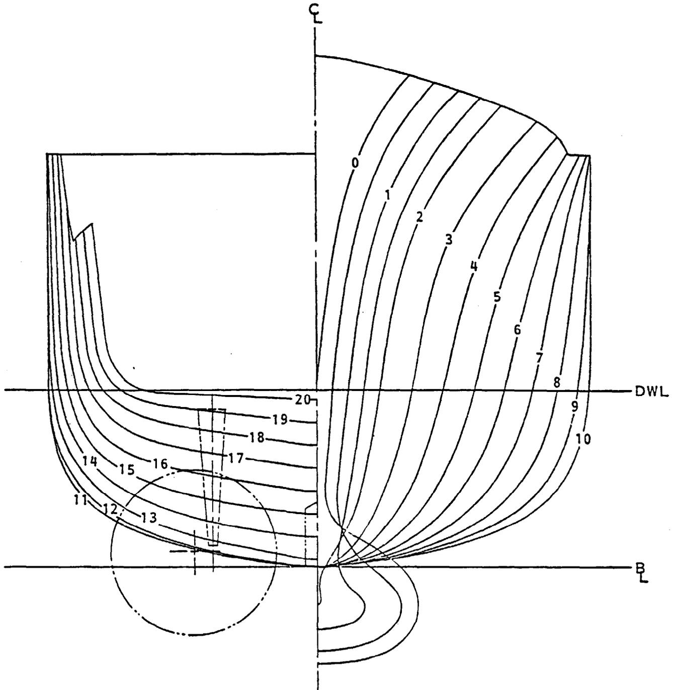
Figure A-1.5 - Body Plan of DD-963 Hull Form (Model 5359)
