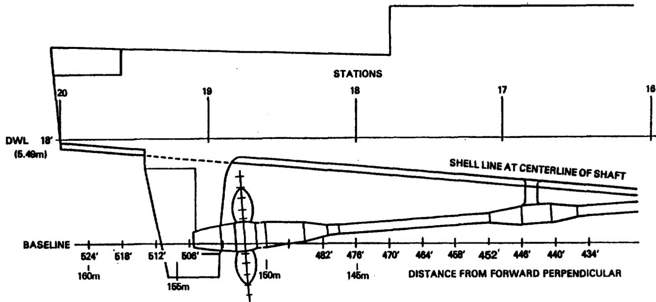
Figure A-6.3 - Stern Appendages of the Bearing-in-Rudder Post Configuration with Controllable-Pitch Propellers - Profile View
