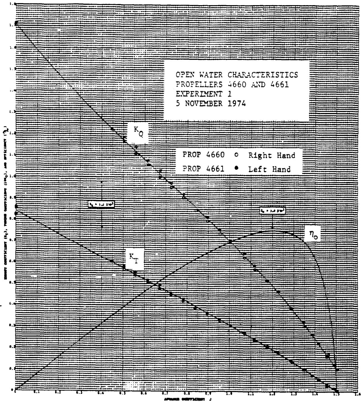
Figure A-1.4 - Open Water Curves for Propellers 4660 and 4661 - DD-963 Design Controllable-Pitch Propellers
