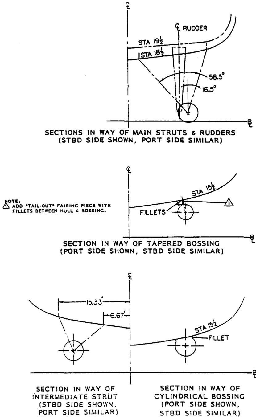
Figure A-4.5 - Stern Appendages of the Twin Shafts and Struts Contra-rotating Propeller Configuration - Sectional Views, from Tomassoni and Slager (1980)
