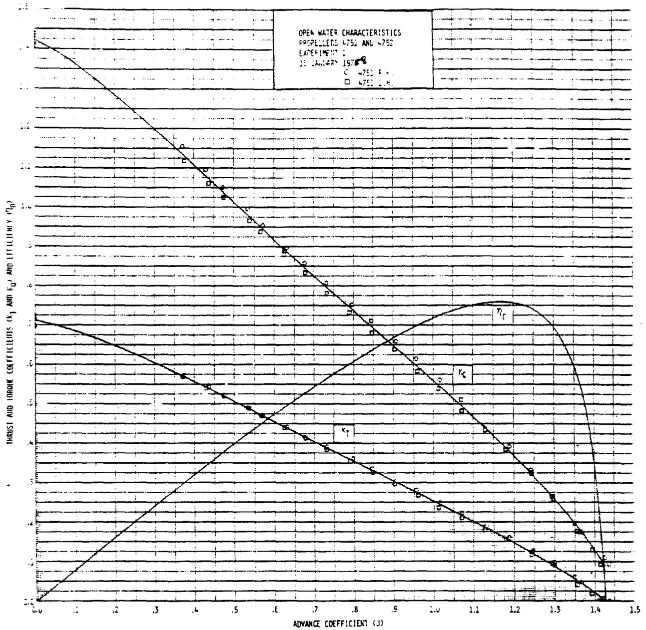
Figure A-10.3 - Open Water Curves for Propellers 4751 and 4752
