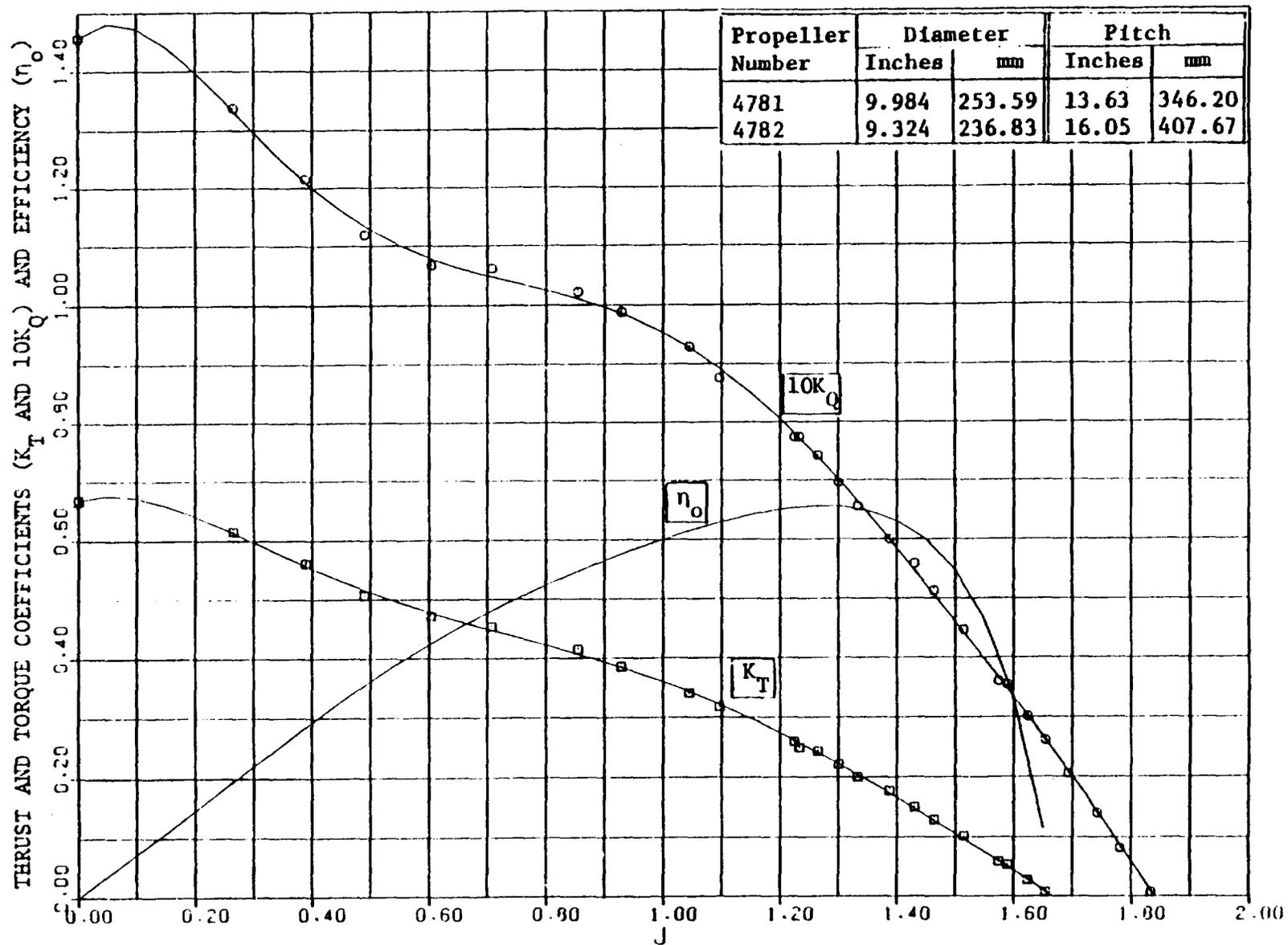
Figure A-13.2 - Open Water Curves for Tandem Propellers 4781 and 4782
