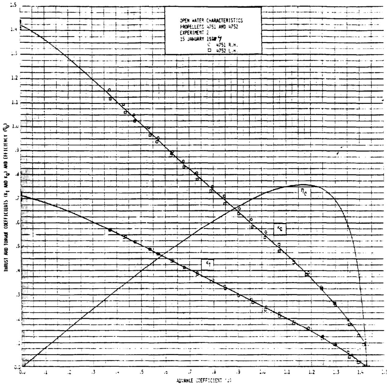
Figure A-7.3 - Open Water Curves for Propellers 4751 and 4752
