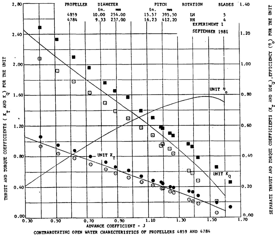
Figure A-12.3 - Open Water Curves for Contrarotating Propellers 4859 and 4784
