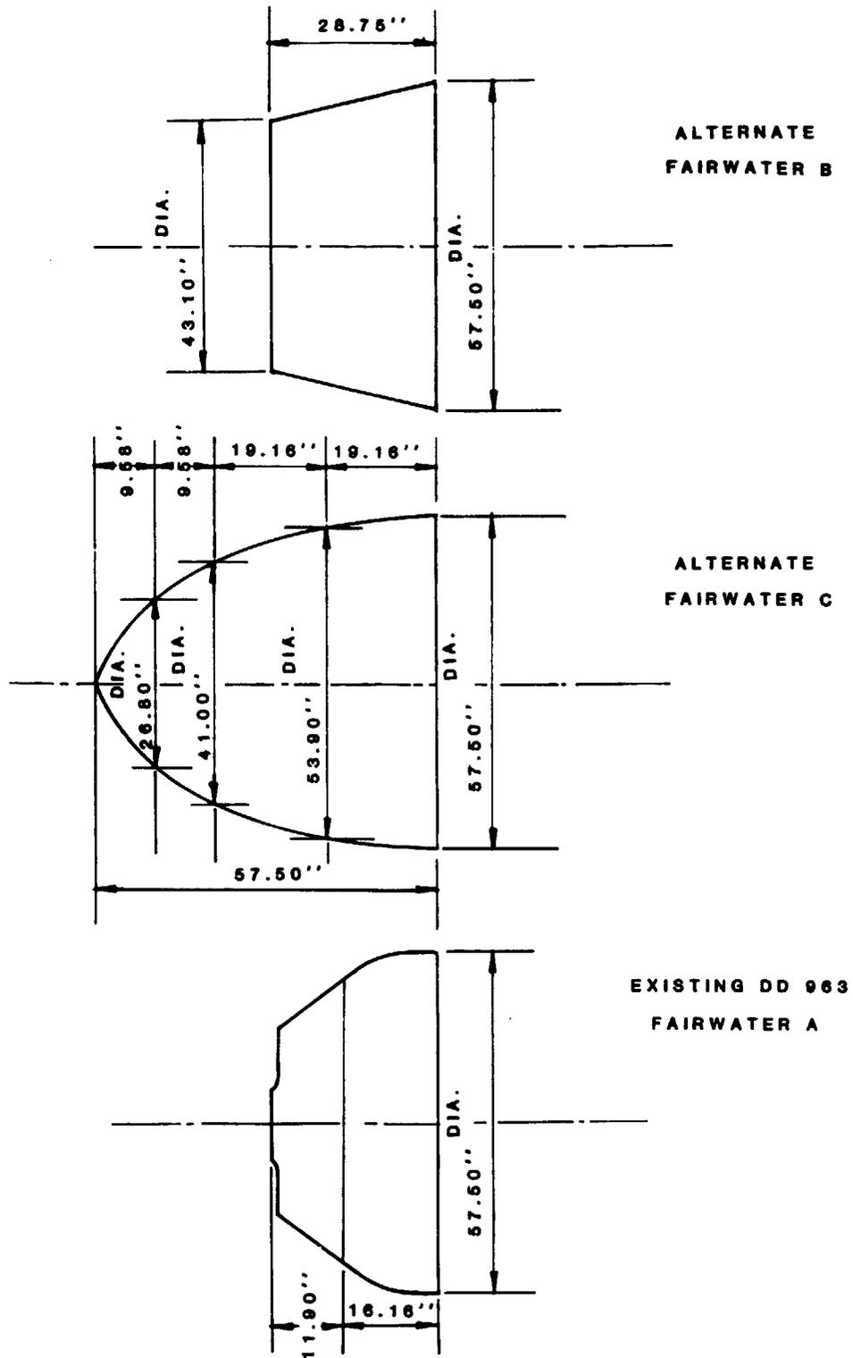
Figure A-9.3 - Details of the Existing DD-963 Fairwater Design (Labeled A) and Those of Two Alternate Low Drag Fairwater Shapes
