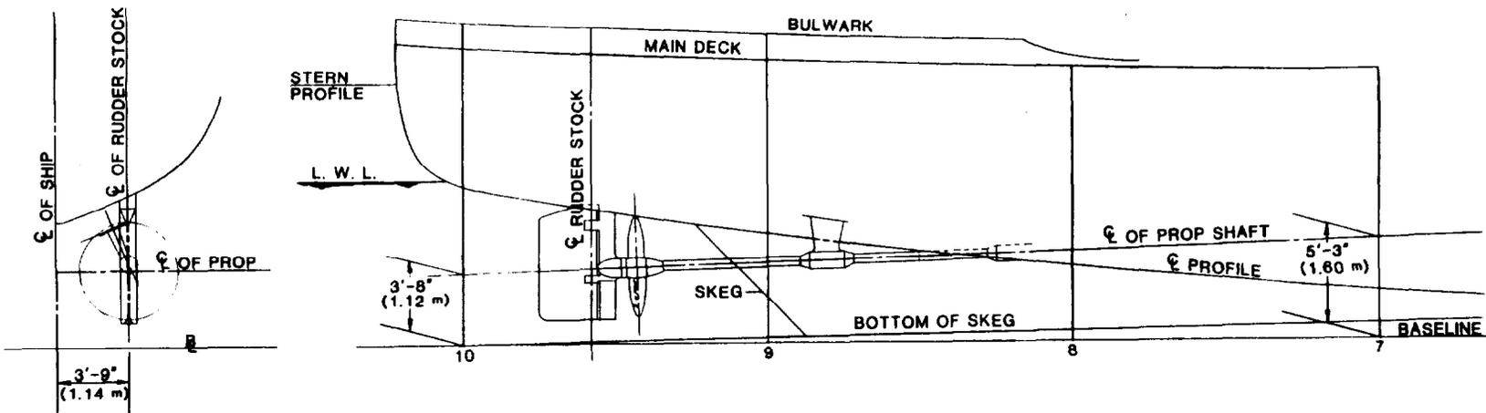
Figure E-1 Stern Appendages of the Bearing-in-Rudder Post Configuration Fitted on a 165-Foot Coast Guard Patrol Boat, Model 3076
