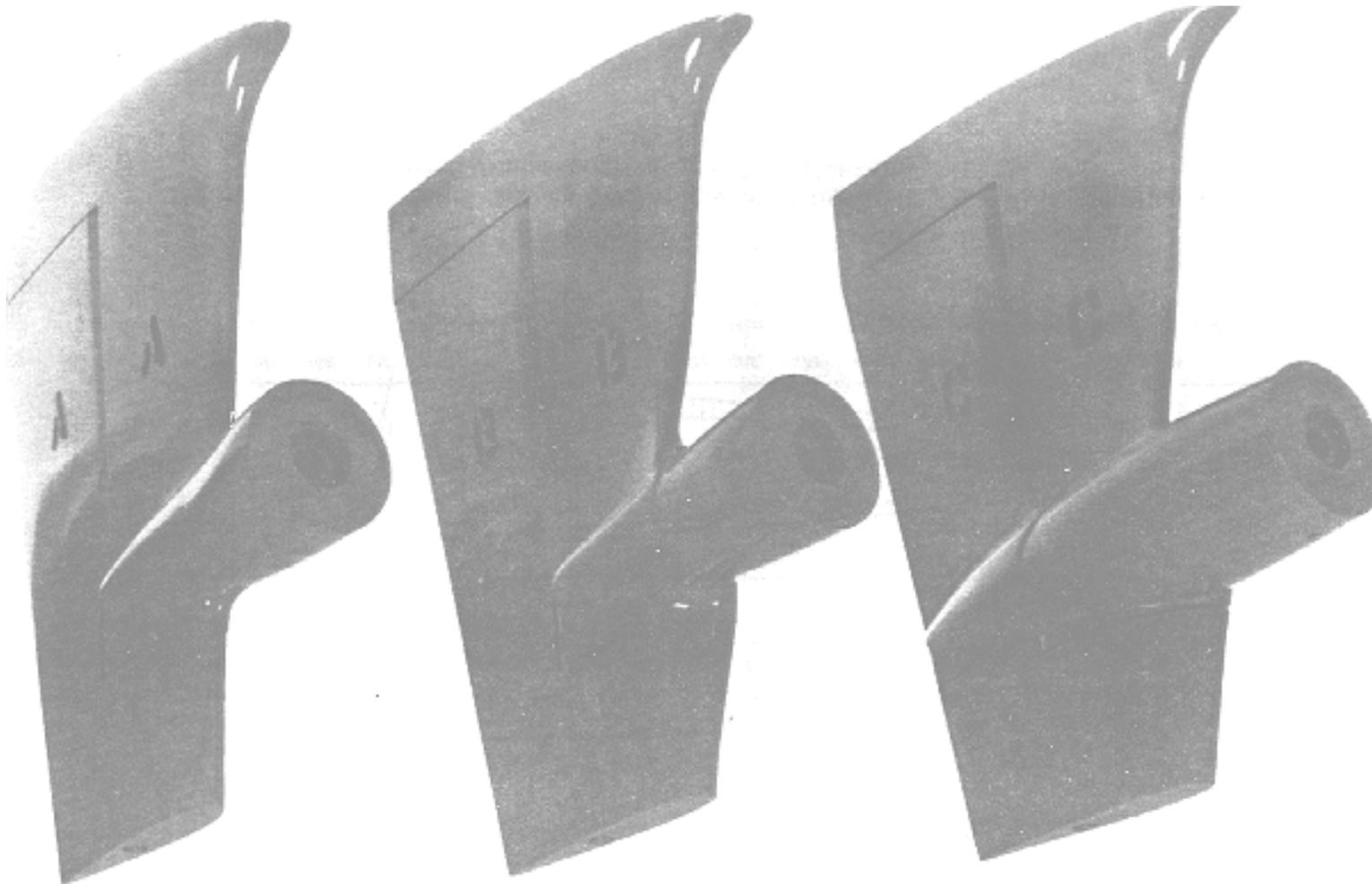
Figure A-6.4 - Photographs of Three Experimental Horn Rudders for the Bearing-in-Rudder Post Configuration with Controllable-Pitch Propellers
