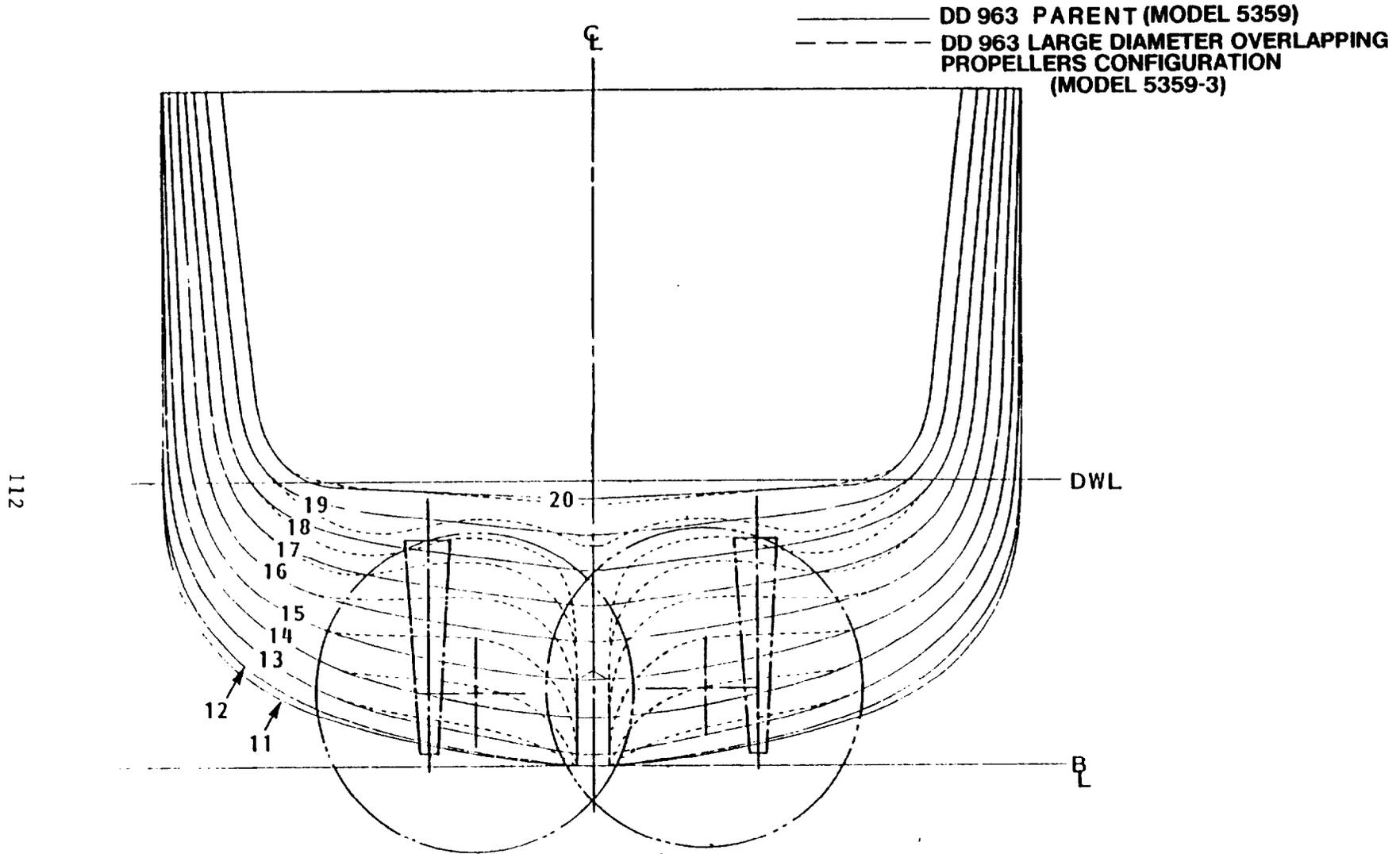
Figure A-10.4 - Comparison of Afterbody Sections of the Large Diameter Overlapping Propeller Configuration and the Parent DD-963 Hull Form, from Tomassoni and Slager (1980)
