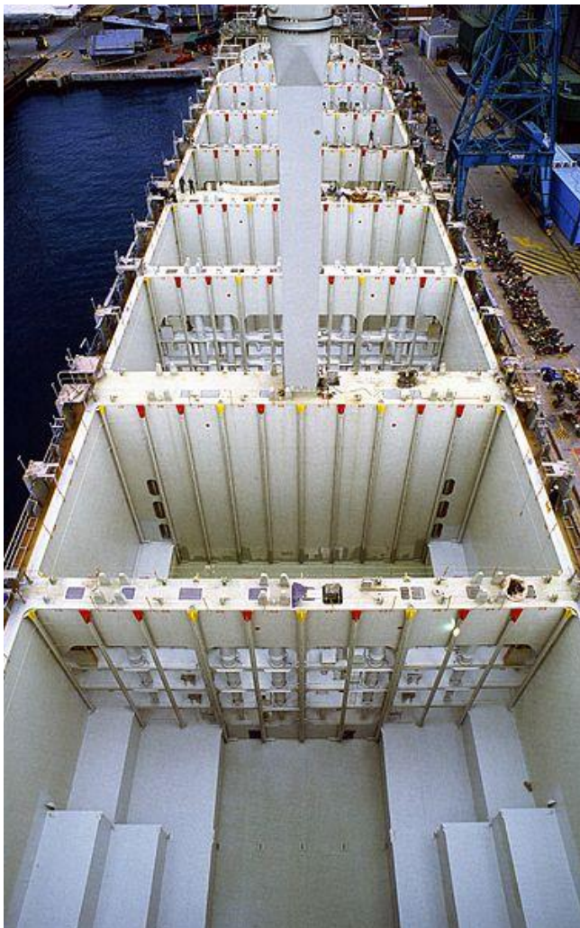
Figure 4: Cell Guides in a Container Ship http://en.wikipedia.org/wiki/File:Containerlader%C3%A4ume_Schiff_retouched.jpg
