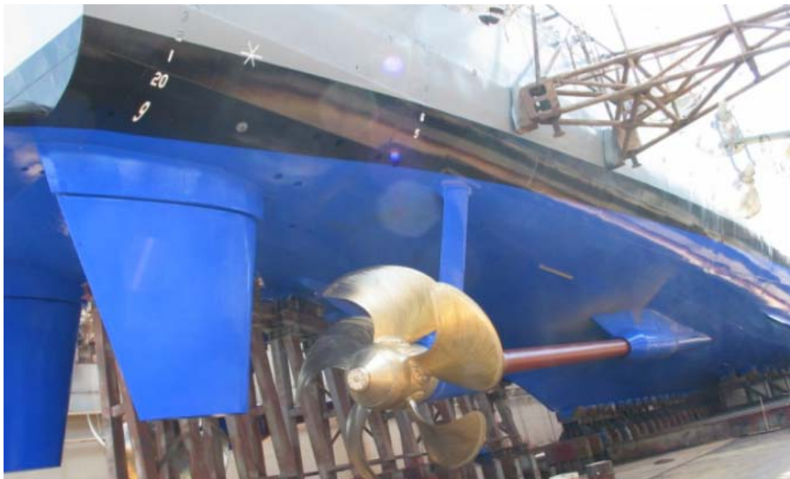
Fig 8 U.S.S. COLE (DDG 67) with fuel efficient underwater hull coat paint
