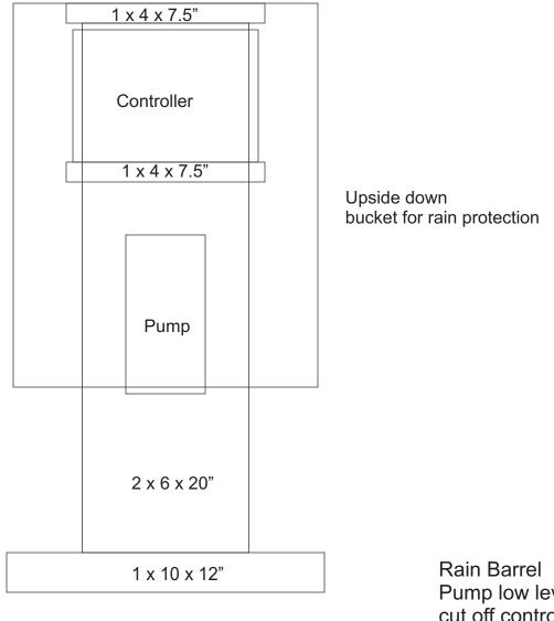
Rain Barrel Pump low level cut off controller Norbert Doerry June 12, 2013
